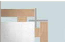
open corner with standard aluminium end plate
