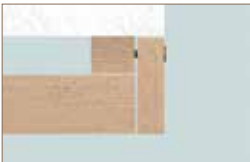
covering the hollow chamber with end plate
