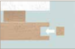
closing the ends with end plate (prior milling of a groove is required)
