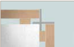
open corner with standard aluminium end plate
