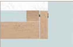
covering the hollow chamber with end plate
