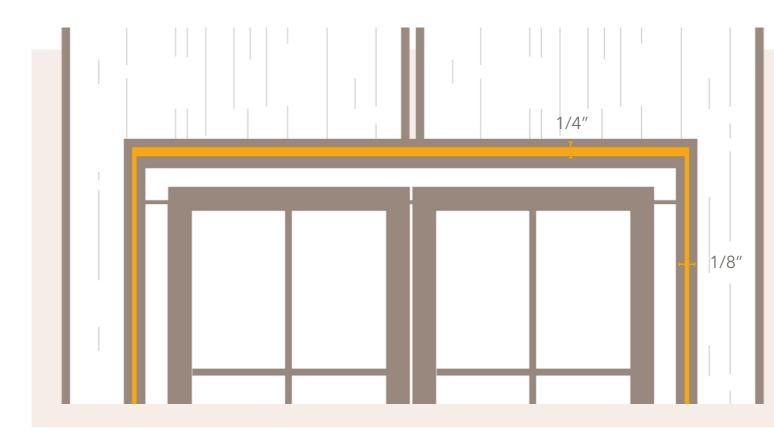
Allow a ¼" gap above windows. Do not caulk the gap above windows (to allow for drainage).
