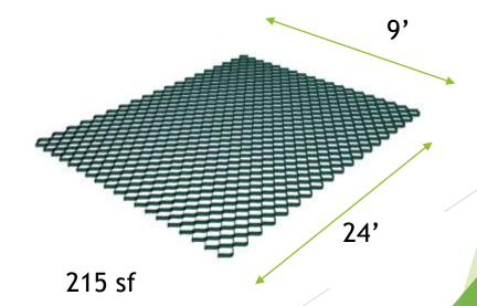
To expand grid to 9' x 24' you will need about 16 pcs. of rebar to aid in the process of full expansion. If you are using rebar J hooks in your installation you can use those instead.
