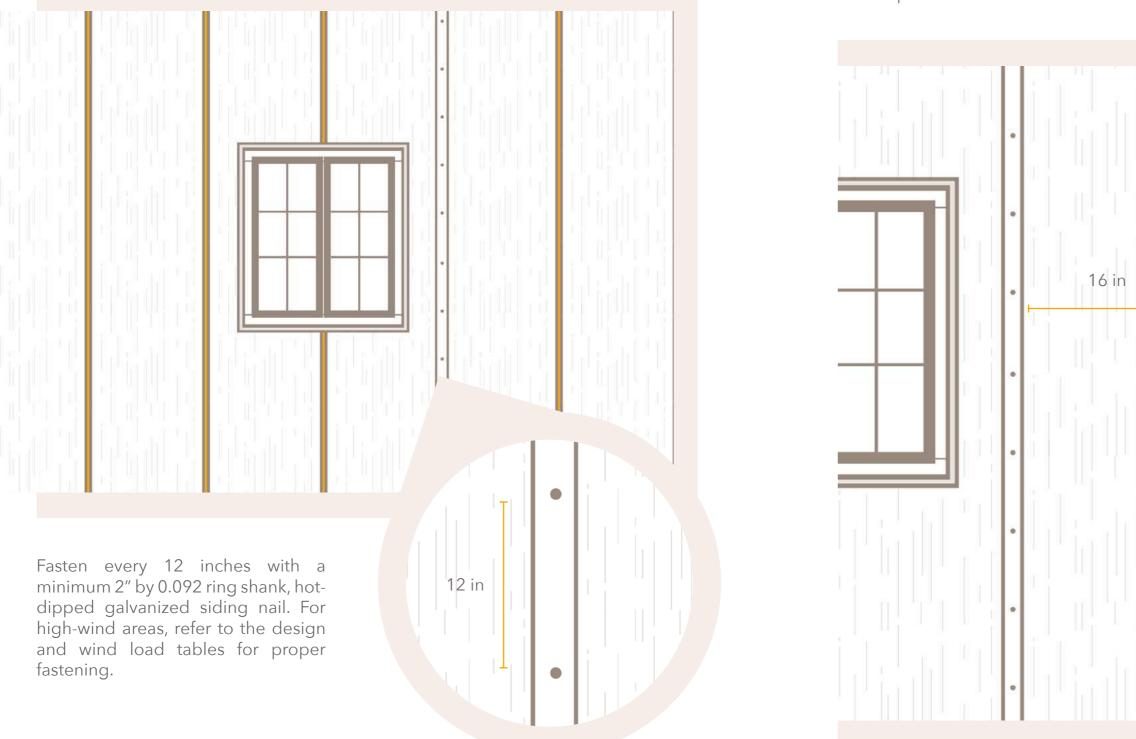
battens are spaced no more than 16" apart.
