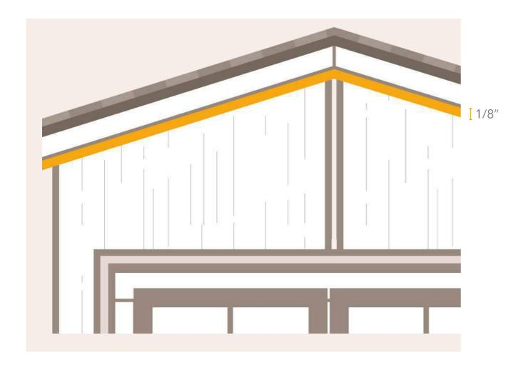
If you choose to skip the band board, extend the corners and battens to the top of the underlying sheets and make sure to use appropriate flashing. Do not bridge floors. Break trim and battens at the subfloor.
