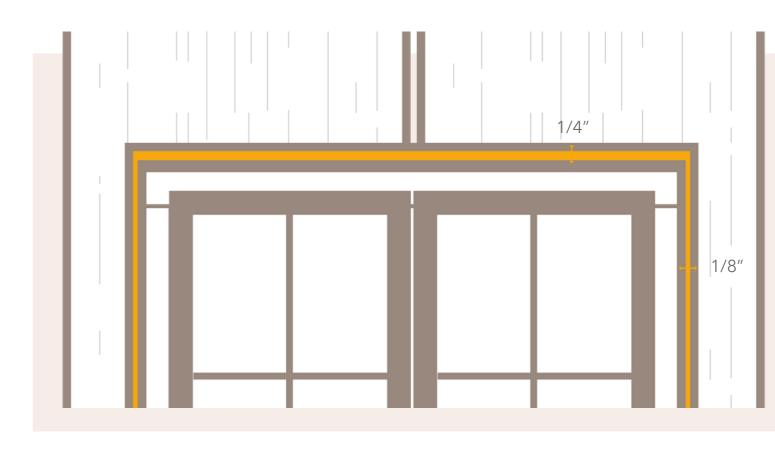
Allow a ¼" gap above windows. Do not caulk the gap above windows (to allow for drainage).
