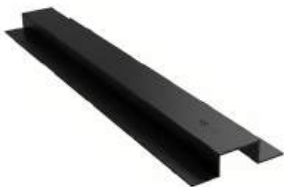
HTC1210BA Facade Hat Channel Black (W x H x L) 1/2" x 1 1/2" x 10'
