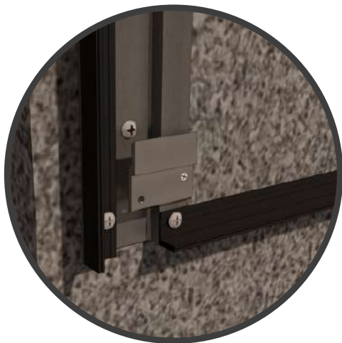
ISOMETRIC VIEW DETAIL 1 Horizontal Wall Cladding HF-Clip Quik-Trim System
