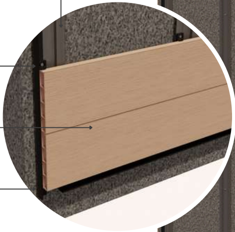
FRONTSIDE ISOMETRIC DETAIL Horizontal Wall Cladding HF Long Clip Quik-Trim System
