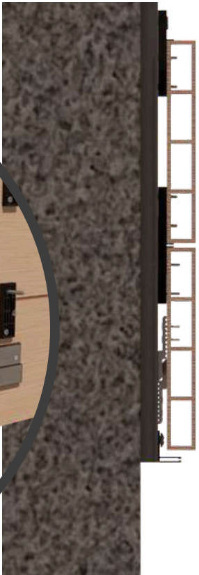
SECTION Horizontal Wall Cladding HF-Clip Quik-Trim System
