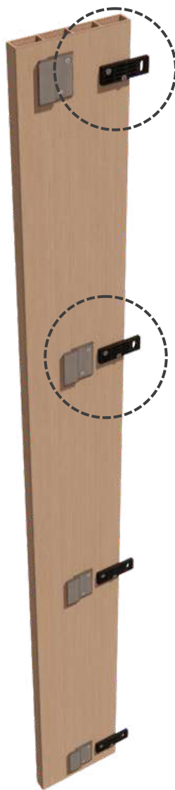
BACKSIDE ISOMETRIC VIEW Vertical Wall Cladding HF-Clip Quik-Trim System
