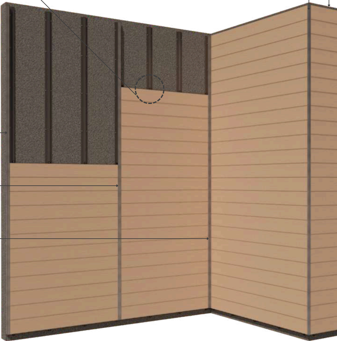
ISOMETRIC VIEW Basic Parts of Cladding HF-Clip Quik-Trim System
