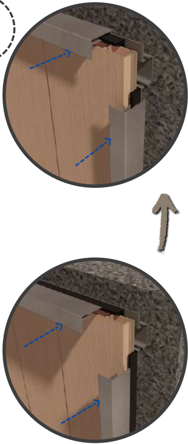
Install the Quik-Trim J-Mold & Quik-Trim Windows J-Mold into the PVC Base
