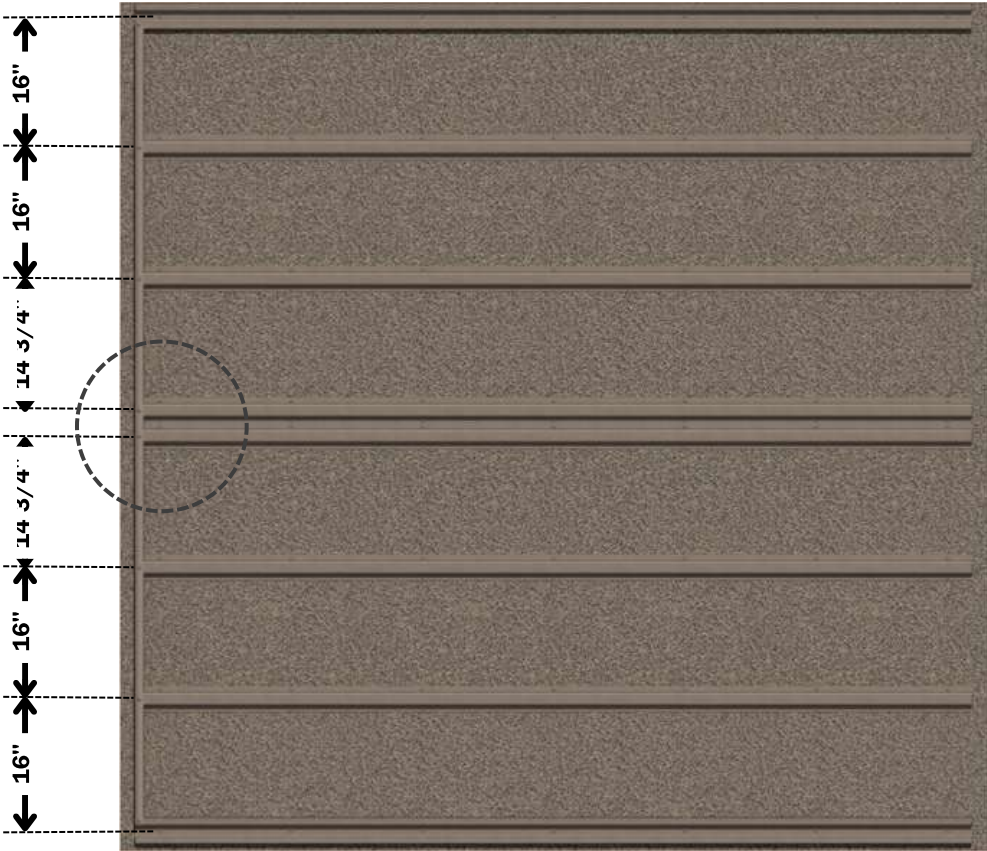
FRONT ELEVATION Deco Profile Quik-Trim System
