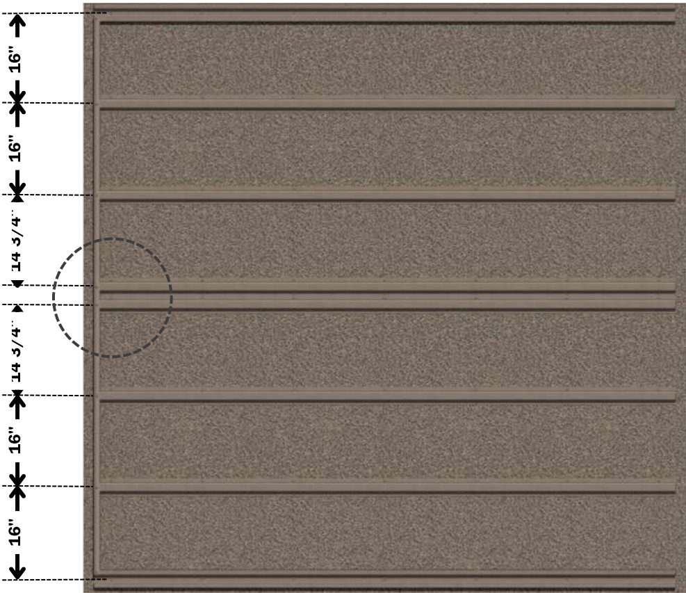
FRONT ELEVATION Siding 12" Quik-Trim System
