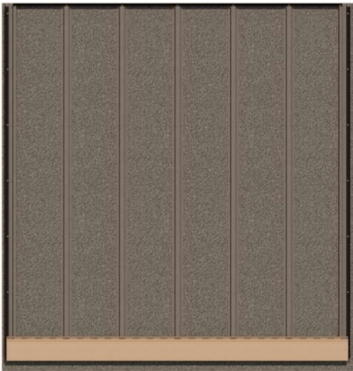
FRONT ELEVATION Siding 6" & 4" Quik-Trim System
